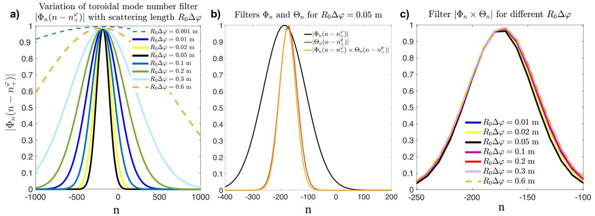
**Figure F3.** (a) Shape of toroidal mode number filter  $|\Phi_n|$  (absolute value) for different toroidal length values  $R_0\Delta\varphi$  of the scattering volume. (b) Comparison of toroidal mode number filters  $\Phi_n$  and  $\Theta_n$ . (c) Comparison of the total effect of a varying toroidal length of the scattering volume  $R_0\Delta\varphi$  on the total product toroidal mode number dependence of the scattering matrix  $U_{np}$ , given by the product  $\Phi_n \times \Theta_n$ .
